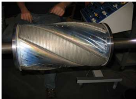
Stabilizers and other complex shapes can be addressed by precision CNC equipment
