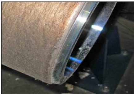
Slip on wearbands welded with minimal distortion
