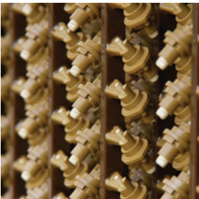
Assembled components ready to be dipped; very precise internal geometry is realized with a ceramic core.
